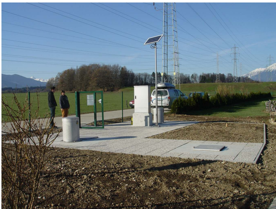
Slika 1. Novo merilno mesto za spremljanje režima podzemne vode v Naklem; foto: V. Savić Figure 1. New measuring station for groundwater regime evaluation in Naklo; Photo: V. Savić
